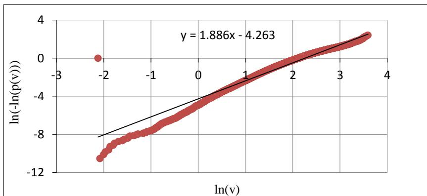
Fig 12 Graphical determination of Weibull parameters for Asabah city
