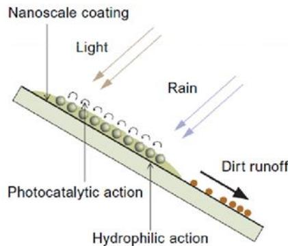
Figure 8. Self-cleaning II – photocatalytic nanotitanium dioxide (TiO<sub>2</sub>)
