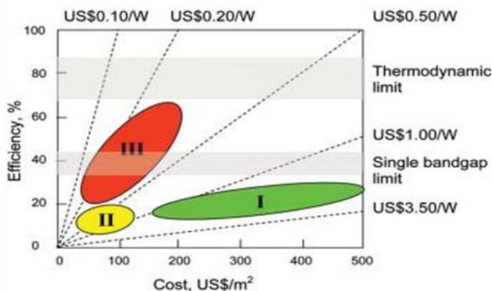
Figure 10. Efficiency and cost projections for first-, second-, and third-generation photovoltaic technology (wafers, thin films, and advanced thin films, respectively)
